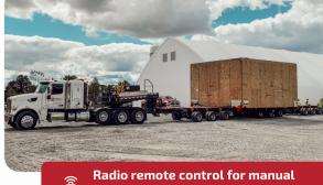
Radio remote control for manual steering of the rear axles under limited conditions at low speed.
