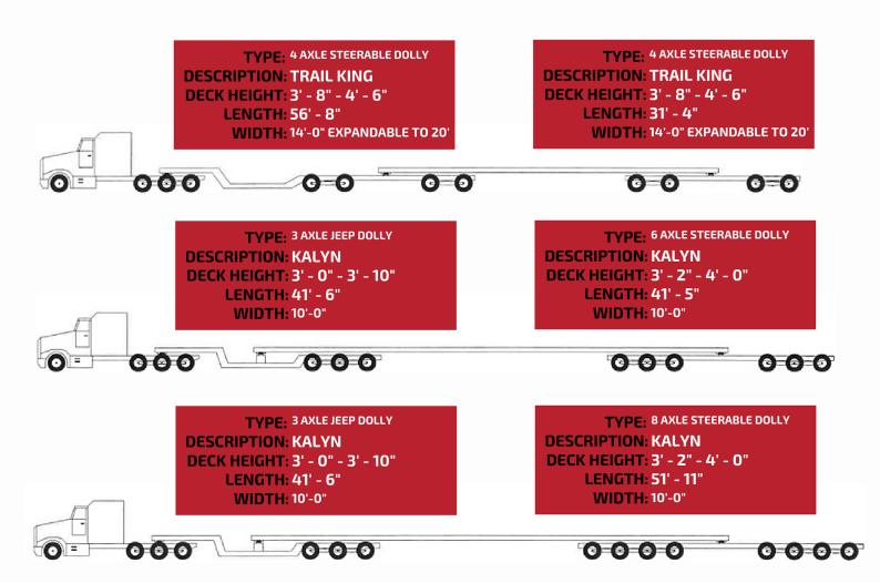
These versatile dollies can be used with multiple manufacturer setups, replace standard wheel area for a steerable axle configuration of your choice, or can be used in combination with a Jeep/Dolly for Bunk work. Our dollies' designs allow for better maneuverability for a greater steering angle, tighter corners and less manual steering. Not to mention they offer remote wireless manual steer and auto alignment after manual steer for an automatic self-centering function.
